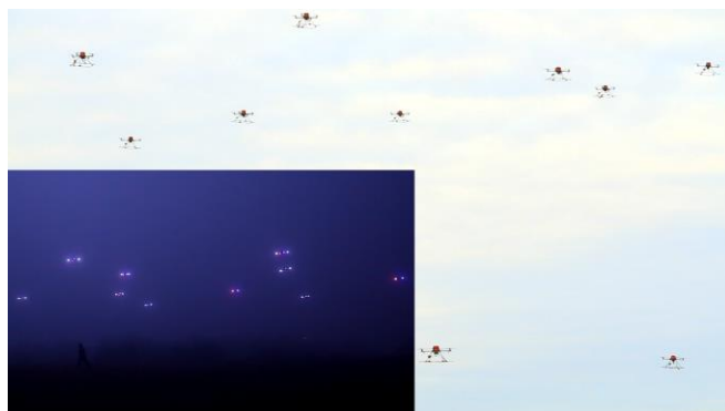
Figure 4. Snapshots of quadcopter flocks of 10 units. Nightlight image: robots are following a target in a grid formation ( r_0 = 6 m, v_0 = 3 m/s). Daylight image: SPP model ( r_0 = 10 m, v_{flock} = 2 m/s).
